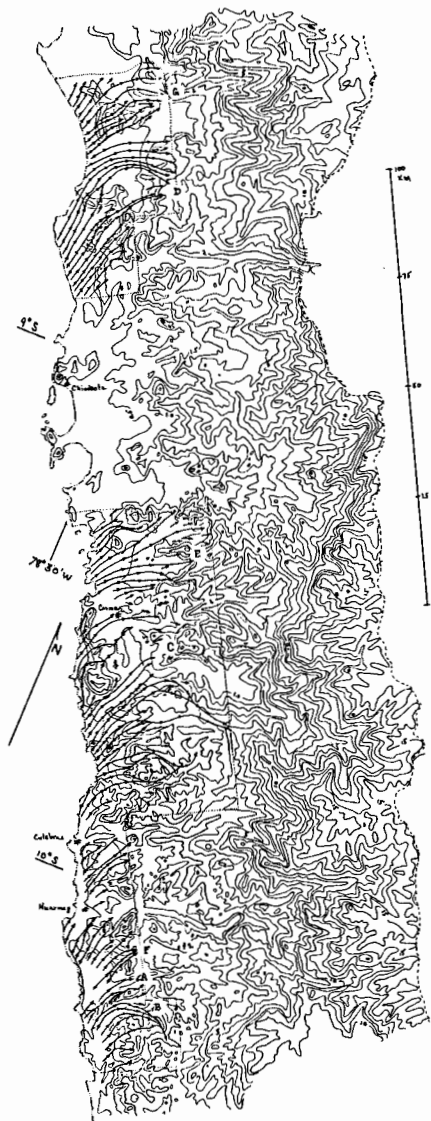
Figure 1. Map of the Peruvian coastline between Trujillo and Huarney showing paths of net sand transport. Contours in feet x1000, with 500 ft contour interval below 2000 ft and 1000 ft interval above 2000 ft. Dashed lines show crest of first Andean summits (Cordillera Negra). Dotted lines show limits of areas mapped from aerial photography. Part of southern mapped area is shown in Figure 2, and the northern mapped area corresponds to Figure 3.
