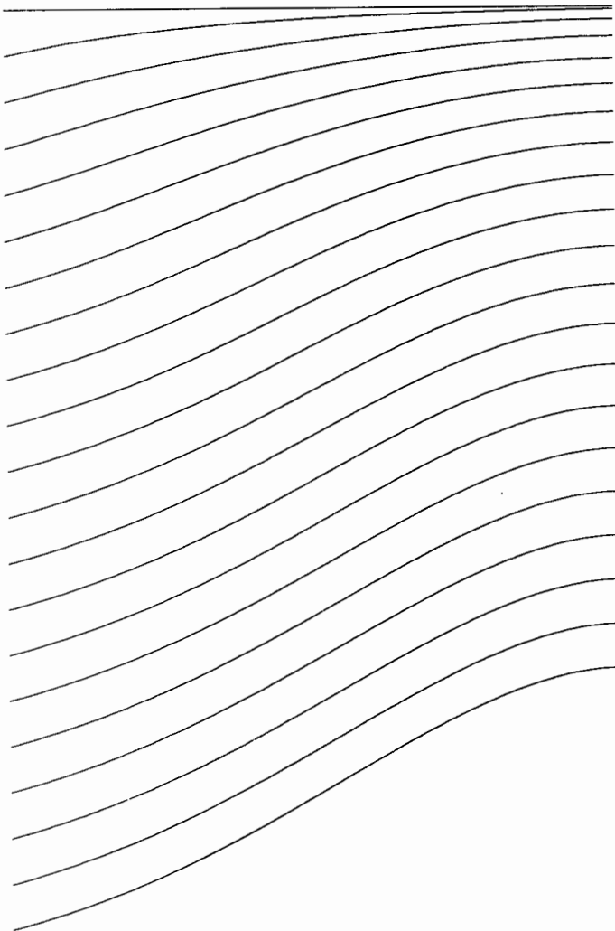
Figure 3.7. Evolution of a two-dimensional slope eroded partially by creep and partially by slopewash. Creep is the dominant process near the divide and slopewash predominates on the lower slope, with the changeover of relative importance occurring near the slope inflection
